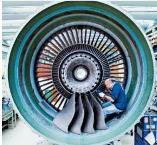
Conventional engine blades are made up of many individual parts.
