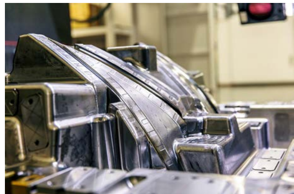
The fully digital 3D laser engraving allows almost unlimited design options on individual surfaces, such as on molds for automotive parts.
