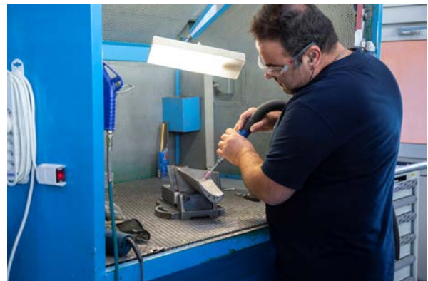
Giuseppe Ballarino works in the Finishing Department at GF Precicast, where the cast components are deburred and polished.
